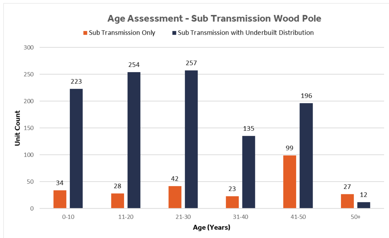
Figure 4-3: Sub-Transmission Wood Poles Age Demographic
